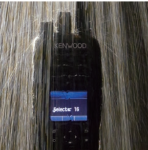
Heavy Rain Test
