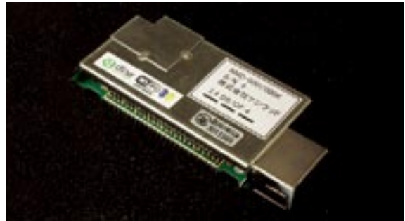
Compact data communication module in compliance with the DLNA guidelines
