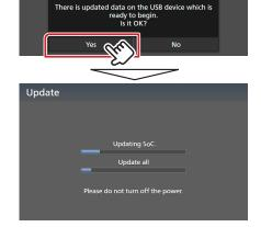
**Caution:** The screen may go blank for a few seconds. Do not unplug the USB memory or Power Off the unit during the Update Procedure.
