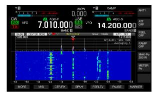
Fig. 87 Example of a Waterfall View
