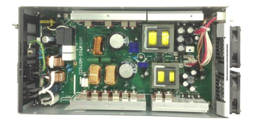
Fig. 43 High-Efficiency Large-Capacity Power Supply
