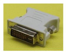
Fig. 140 DVI (Male) - VGA (Female) Conversion Connector (Commercially Available)
