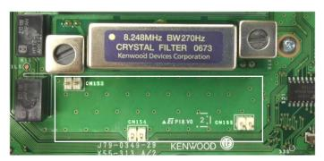
Fig. 16 Additional Roofing Filter Mounting Slot
