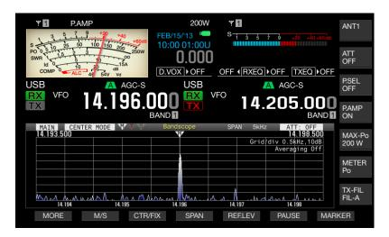
Fig. 112 CW Auto Tuning Activated with a Long Touch
