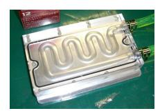
Fig. 5 Water-Cooling Head
