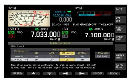
Fig. 104 Modulation Source Screen
