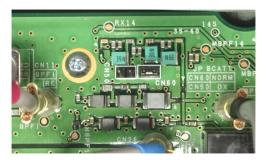
Fig. 24 Main Band Jumper Pin Locations
