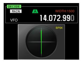
Fig. 100 Vector Scope (PSK Mode)
