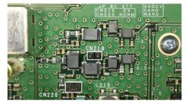
Fig. 25 Sub Band Jumper Pin Locations
