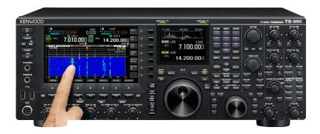
Fig. 94 Touch Screen (Touch-controllable Main Screen)
