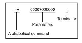
Commands can be classified as shown below: Set command (sets a particular Input command condition) (input to the transceiver) Read command Computer (reads an answer) control commands Output command Answer command (from the (transmits a transceiver) condition)
