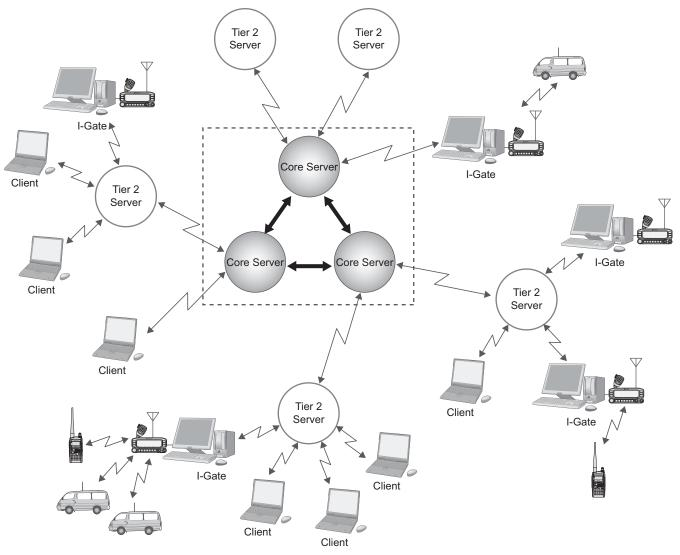
Figure 7-1 APRS Network Conceptual Drawing
