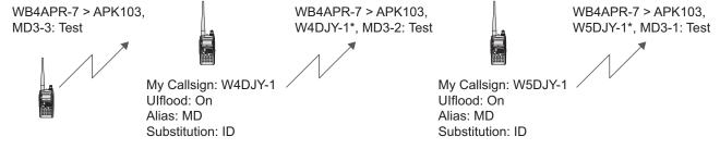
Figure 7-6 Using UIFLOOD
