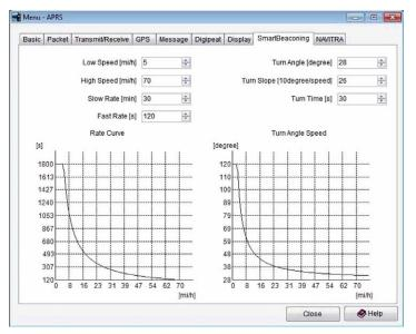
Figure 8-11 Graphs of SmartBeaconing
