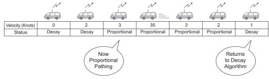
Figure 6-3 Switching between Decay Algorithm and Proportional Pathing (when Stopped = 1 (knot); Moving = 3 (knots))
