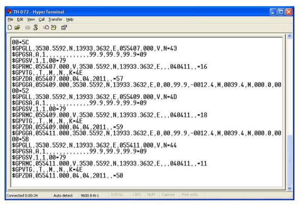
Figure 4-13 Displaying the Raw Data
