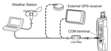
Figure 4-2 Connection Example of GPS Receiver
