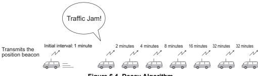
Figure 6-1 Decay Algorithm
