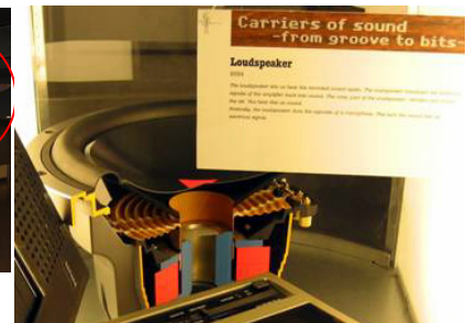
Cross section showing how sound is output
