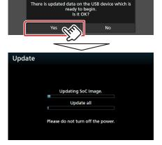
**Caution:** The screen may go blank for a few seconds. Do not unplug the USB memory or Power Off the unit during the Update Procedure.
